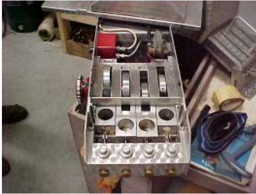
Cam mechanism that allows ball to fall into pocket where it is injected.
